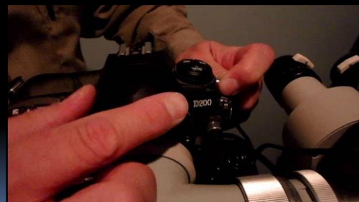
Testing flash synchronization connection between instrument and camera.
