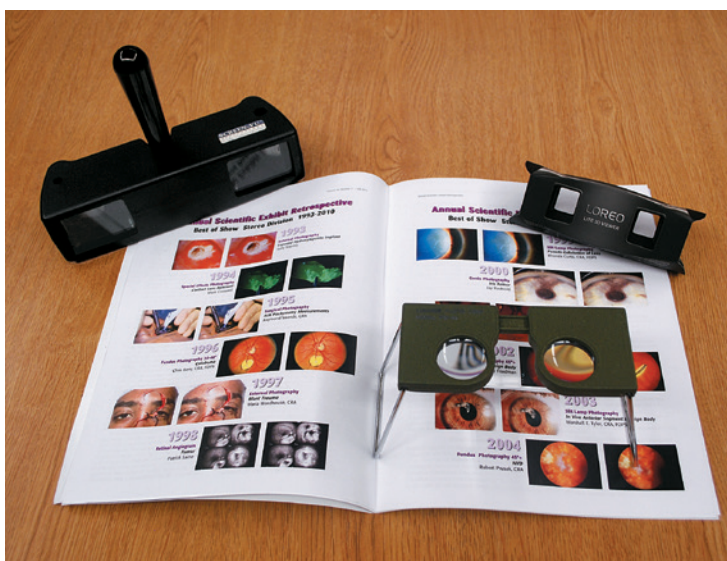
Figure 1: Stereo viewer types, left to right: Wheatstone-type (mirror), Brewster-type (lenticular), Loreo Lite (base-out prisms).
