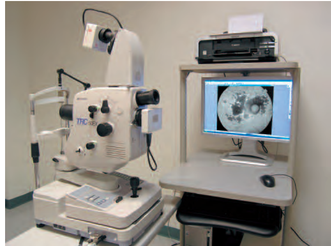
Figure 2: Fundus camera FAF system with monochrome sensor and FAF barrier filter mounted on TV relay lens on top camera port.
